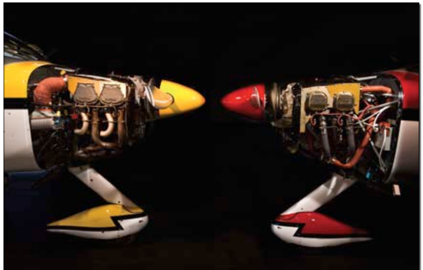
When power matters, go for the big inches. The IO-390 (left) makes 30 horsepower more than the venerable IO-360 parallel-valve engine (right).
