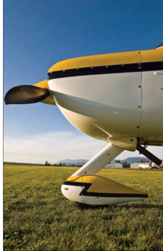
Fitting the IO-390 to the Sportsman airframe required a slightly altered upper cowling. The lower blister allows for efficient cooling flow and shrouds the four-into-one exhaust that most TWTT customers buy.
