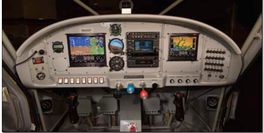
The Sportsman panel is clean, functional and full of goodies. Advanced Flight's EFIS and engine monitor flat screens are a delight.
