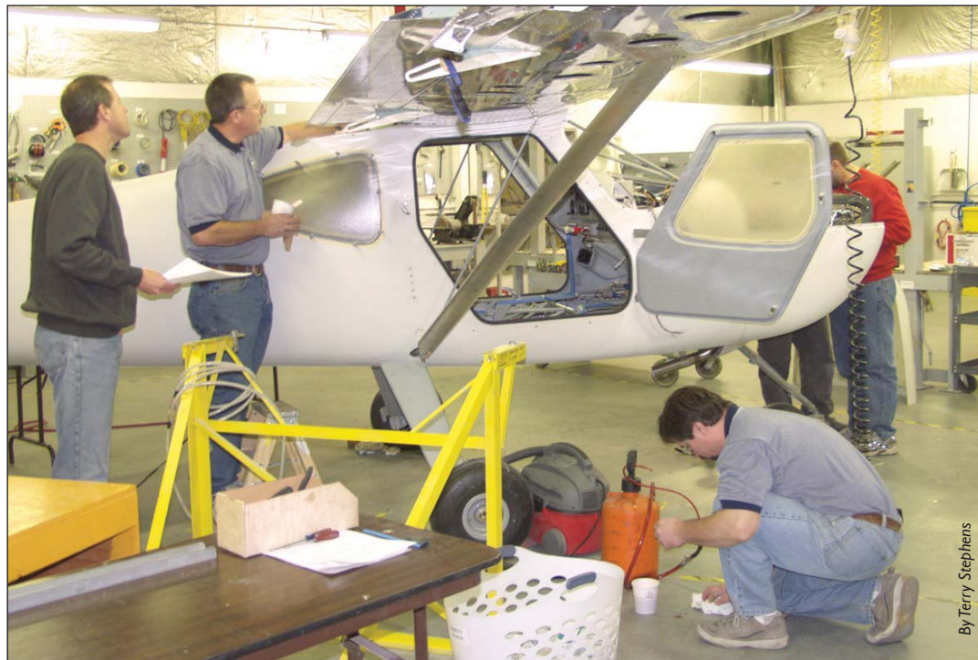
Glasair President Mikael Via (left) oversees work at the Arlington plant on a customer-built Sportsman 2+2. Owners build at least 51 percent of the plane to meet FAA regulations for kit plane construction.
