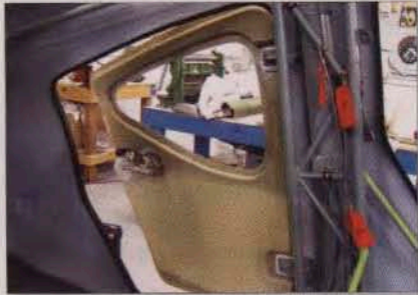
On Day 14, the interior door latch has been installed and aligned.
