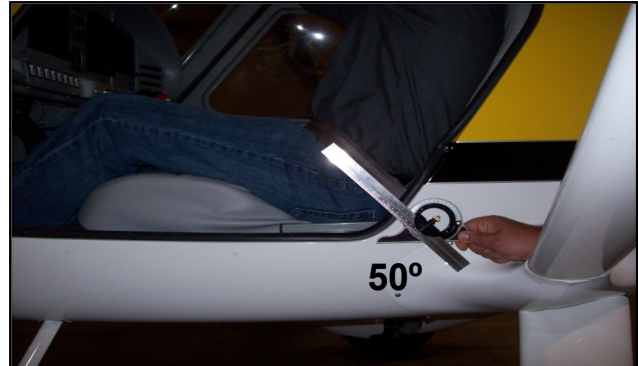
Retrofit (new) configuration: Seat-back in aft position
