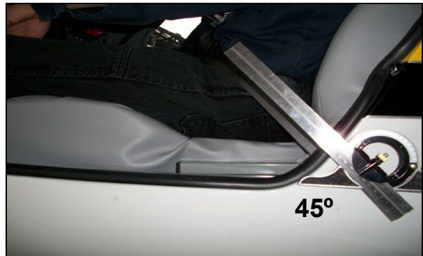
Retrofit (New) configuration: Seat-back in forward position
