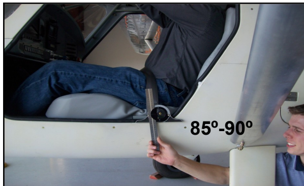
Current configuration: Seat-back in aft position
