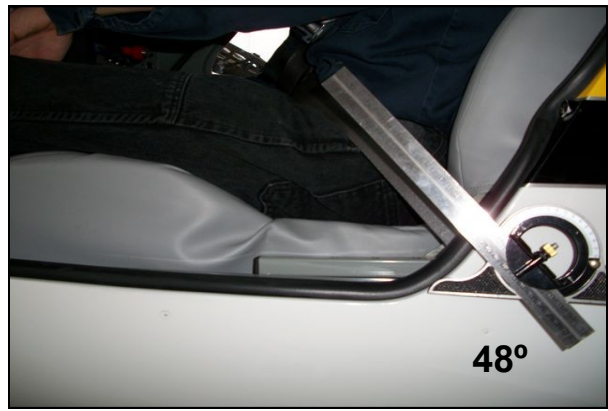
Retrofit (New) configuration: Seat-back in mid-position
