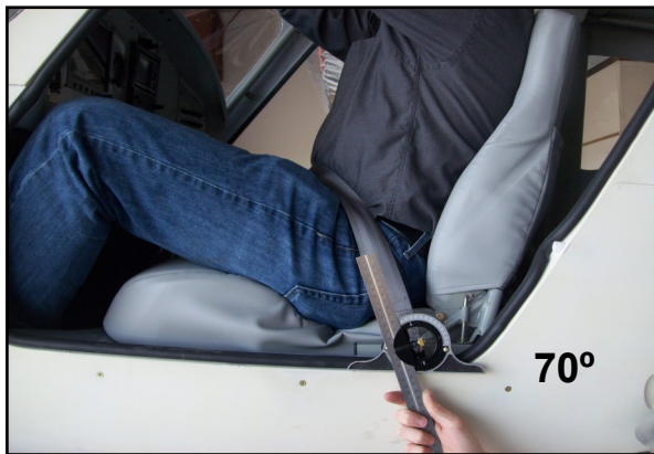
Current configuration: Seat-back in mid-position
