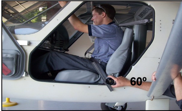
Current configuration: Seat-back in forward position
