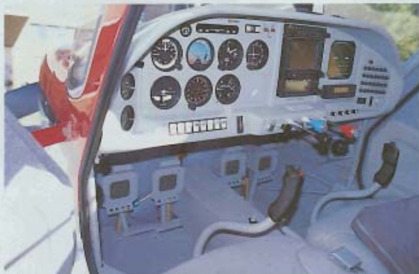
The instrument panel, control sticks and dual rudder/brake pedals are seen in this view.
