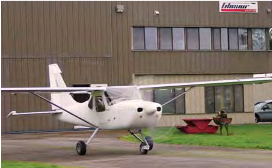
Preparing for first flight, 18 working days after starting the project. This is actually a ground runup test, but the airplane would fly later that day.
